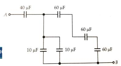
points A and B as shown in Figure. Also calculate the total charge that flows in the circuit when a 100 V battery is connected between the points A and B.
